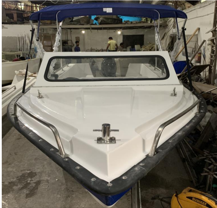
Merlyn with Foldable Stainless steel/ Aluminum structure called Bimini Top
